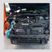
No sufficient space to remove old alternator due to big size
