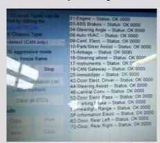
LIN communication is OK (No DTC set by ECU in any electronic system of the CAN due to alternator replacement).
