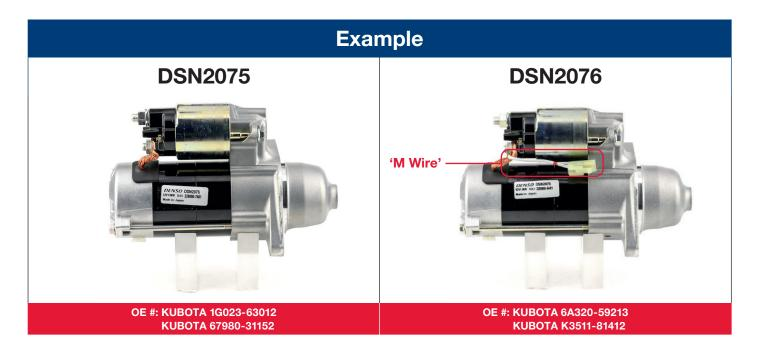
The explanation below describes the difference between the above starters. The difference is that DSN2076 has an 'M Wire' — as indicated (above right) — which is a wire with its connector attached to the motor terminal on the starter solenoid, whereas DNS2075 does not have an 'M Wire'.
