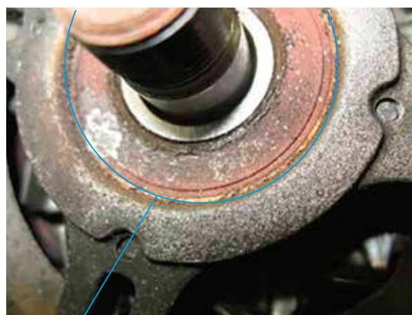
Lagăr frontal defect
