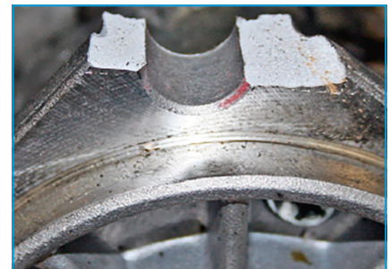
Starter to engine mounting bolt hole broken off due to mishandling, improper installation or over-torquing of the engine bolt.
