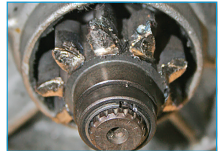
Extreme case of pinion re-engagement.
