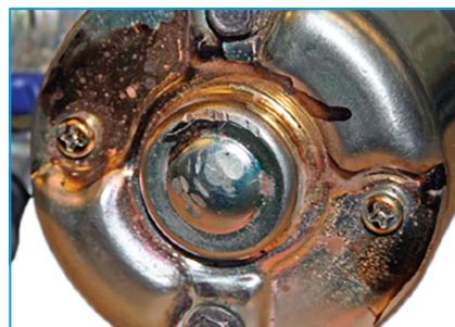
Melted insulation on the starter end housing thru bolts. This is a sign of starter abuse (overheated).
