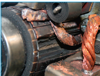
Commutator surface is glazed. Commutator segment bars bent.
