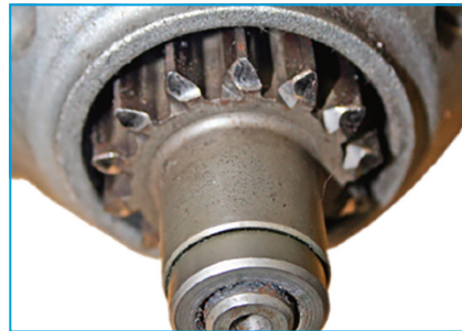
Moderate case of pinion re-engagement.
