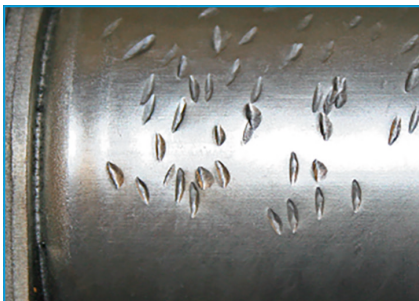
Solenoid cover has been struck repeatedly with a hammer or some other foreign object.
